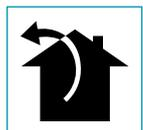
In this version the fumes and vapours are conveyed outside through the exhaust pipe. To this end, the hood outlet fitting must be connected via a pipe, to an external output.
